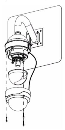
Step 12 Attach the dome assembly by aligning its tab with the opening in the base plate, pressing it into place, and securing the three TORX screws (see Figure 2-12).
